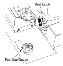
Figure 4-4 Seat Lock Lever
